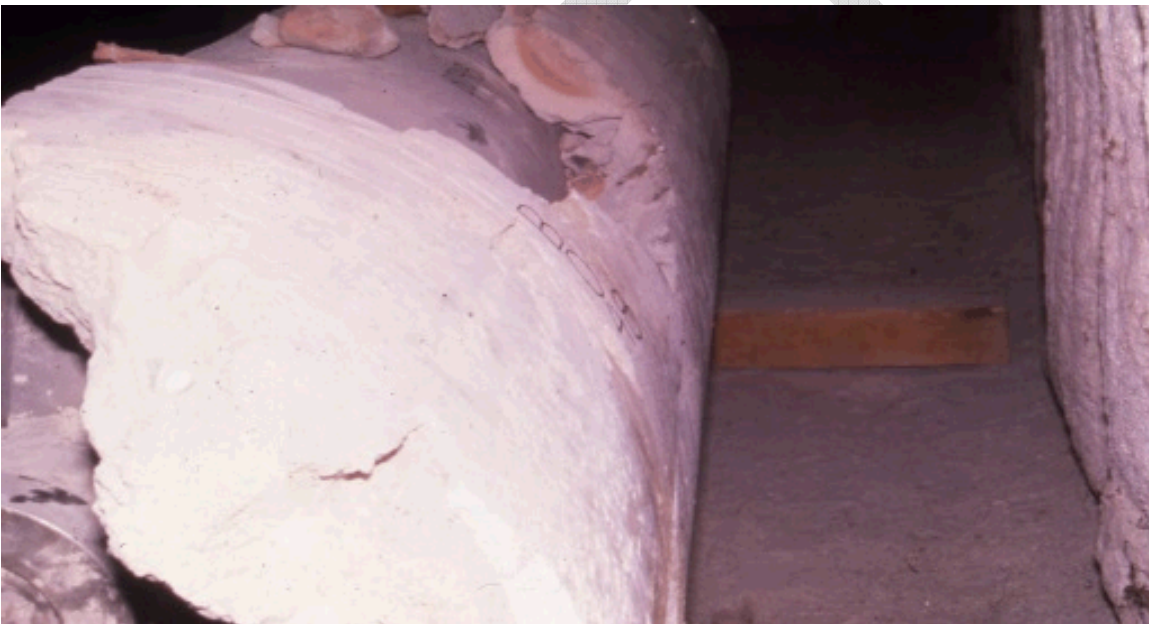
Figure 2.5 WIPP Room B heater with reconsolidated salt caked on the circumference.
